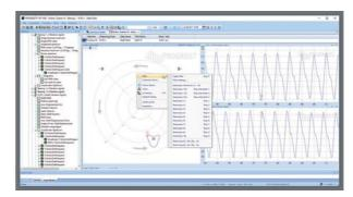
Filtering of shaft orbit
