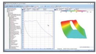
Machine tree, p-V diagram, and p-V diagram trend
