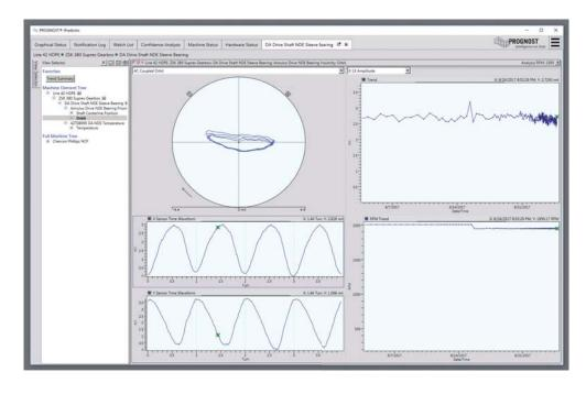
Orbit analyses: These analyses are used for sleeve bearings. It saves startup and coast down events and steady-state operational data.
