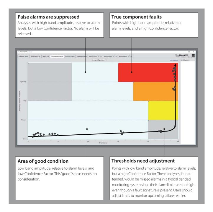
The Confidence Factor and built-in Two Factor Alarm logic have been developed to:
