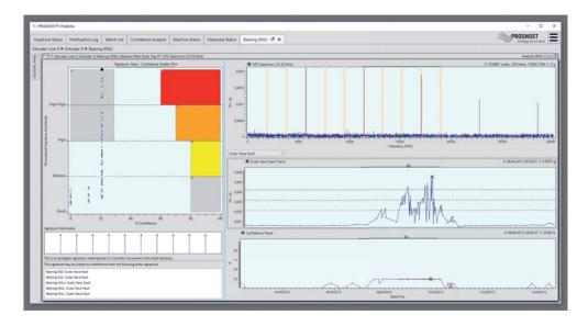
Low Confidence Factor despite of high band amplitude: These amplitudes do not belong to the failure represented by the bands in the upper spectrum since only a few peaks match with this failure pattern.
