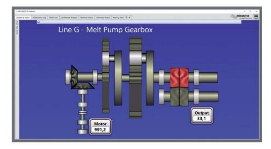
Users check the status of each component through a series of graphics. Components in an alarm state change color to indicate Warning, Alert, and Alarm.
